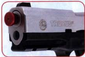
A laser-emitting device like this one from LaserLyte aids dry-fire practice with a carry gun.
